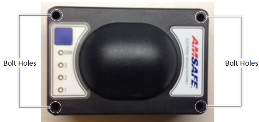
Figure 9. EMA (100) Bolt Holes
