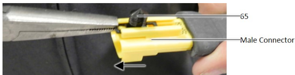
Figure 48. X-Tree Clip (65) Removal
