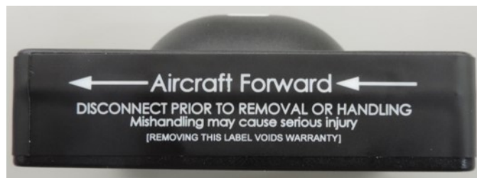
Figure 8. EMA (100) Aircraft Forward Label
