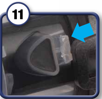
11 Inspect atomizing head for damage or wear which could result in fluid leaks or poor performance.
