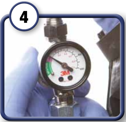
4 Set air pressure at 30 psi for 1 st stage (only air flowing)
