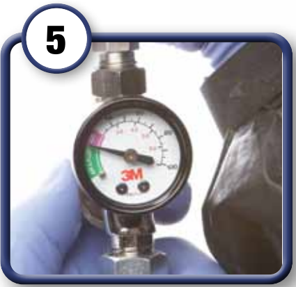
5 Set air pressure at 20 psi for 2 nd stage (air and fluid flowing)
