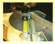
For an <u>outside</u> miter cut you have the wing that is not against the fence pointing toward the back of the saw.
