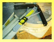
Line the <u>center bar</u> along the table insert or blade to make a miter cut.
