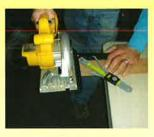
the other wing to the mark for the miter angle. Line blade to mark and use the *Quick Angle®* as a saw guide.
