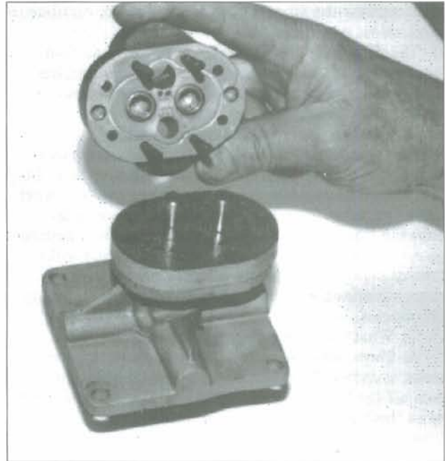
Cleanliness is absolutely essential in a hydraulic pump due to very tight clearances of the pump mechanism.
