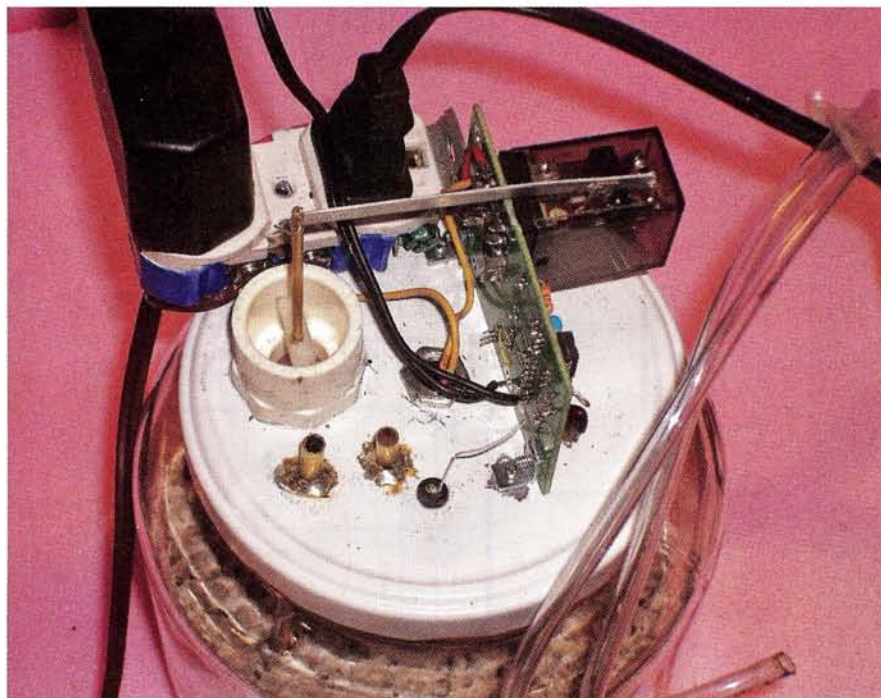
Purge valve control PC board and power supply mount on lid
