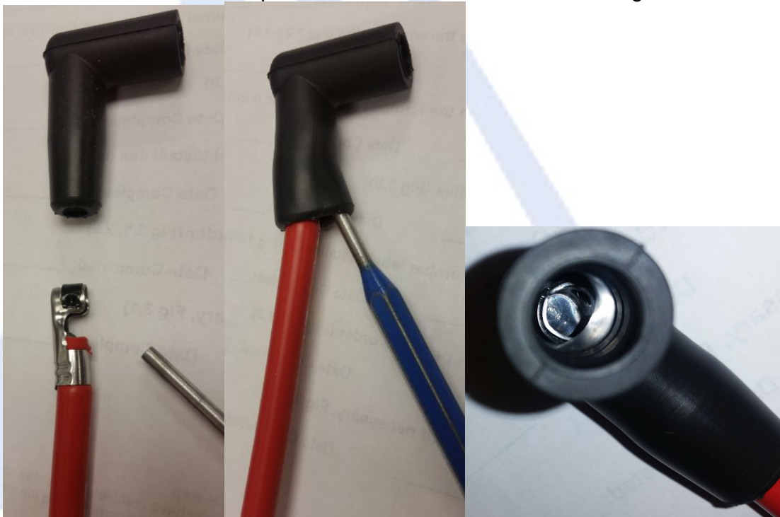
Figure 15: Inserting Terminal into Boot
