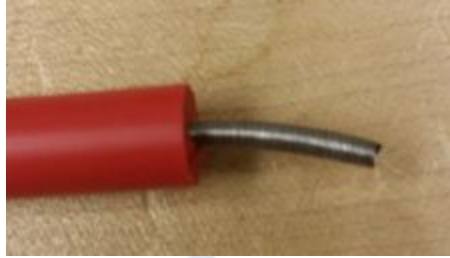
Figure 13: Exposed Core of Spark Plug Wire
