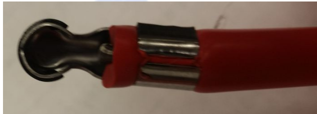
Figure 14: Terminal Crimped with Central Core Folded
