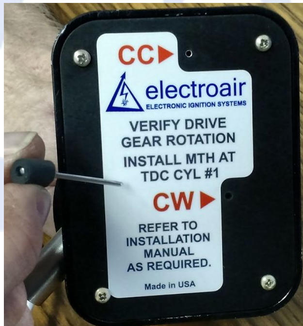
Figure 7: Installation of MTH Alignment Pin
