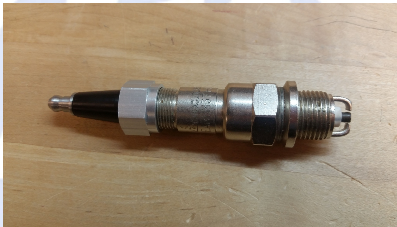
Figure 12: Spark Plug Tower Attached to Spark Plug
