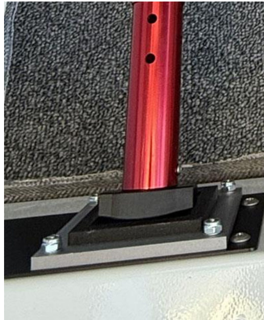
Figure 2: Rudder Lock Base Installation
