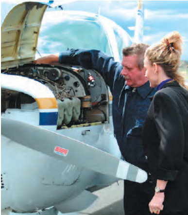
Figure 1-17 The oil quantity should be checked during the preflight inspection prior to every flight.
