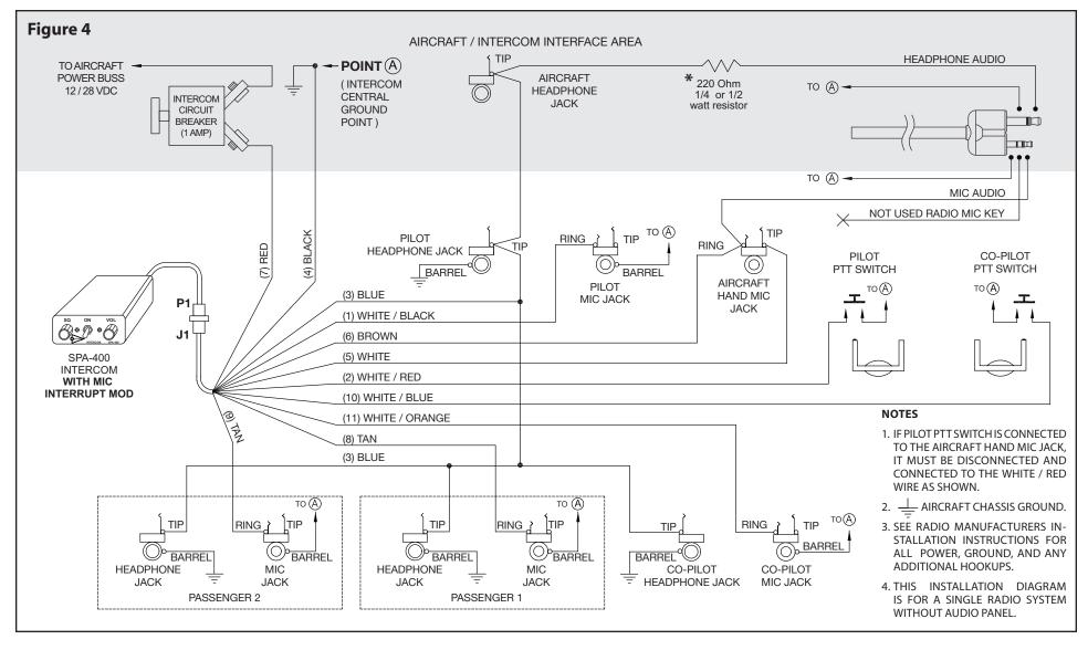
SPA-400 – ICOM A20, A21 Radio Installation Wiring Diagram
