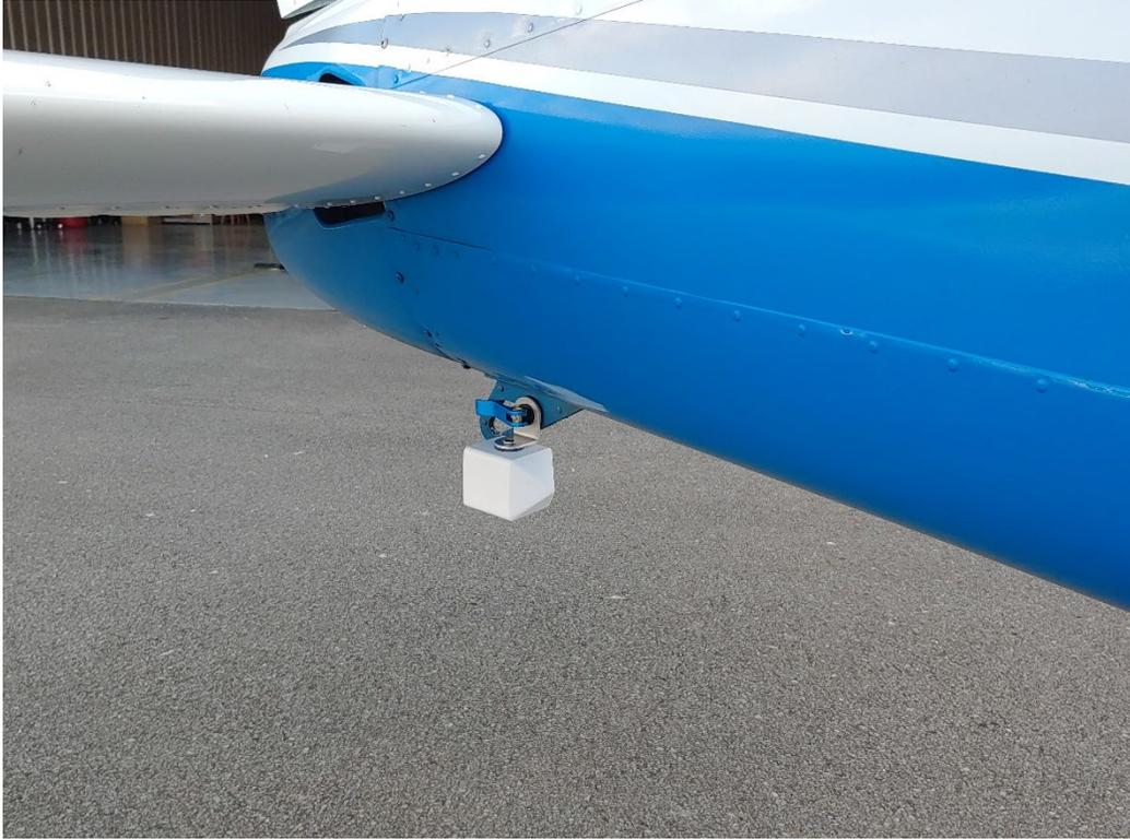
*Figure 8 Stadia correctly mounted to a tie-down ring at the tail*
