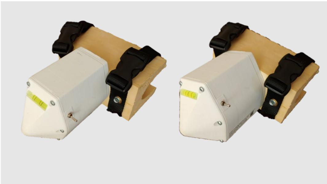
*Figure 5 Stadia showing rotation of the LIDAR unit*
