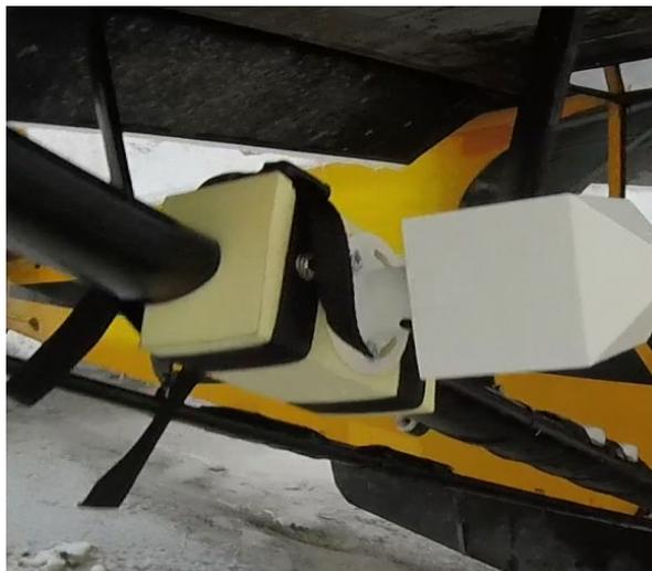
*Figure 6 Previous Stadia model showing correct mounting on wing strut*
