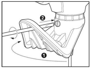
**CAUTION:** Do not remove the screw from the probe stand. Be careful to not overtighten the screw. Always use a screwdriver to fasten screws.
