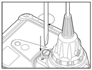
**CAUTION:** Do not remove the screw from the probe stand. Be careful to not overtighten the screw. Always use a screwdriver to fasten screws.
