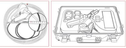
2. Do not roll the probes up too tightly (aim for a diameter of at least 15cm)
