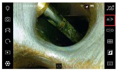
Once the dual view is activated, a line will appear that separates the screen. With the dual view mirror attached, the front view will be indicated by the F letter and the side view by the S letters respectively.
