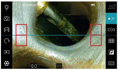
The Line will aid as a border between the two sides of the mirror and ease navigation and orientation.
