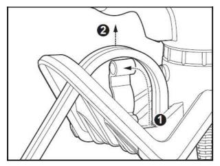
Put down the holder and let the tube hang on to it. Insert the tip end and bending neck through the holder hole above 20 cm. The tube can be fixed.
