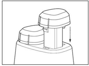
4 Repeat the process and push the new battery into the battery holder of the X750
