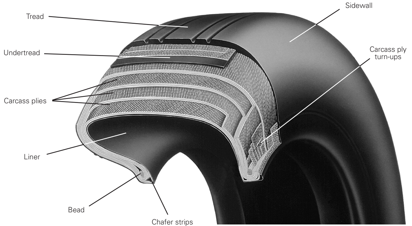
Typical bias-ply tire construction.
