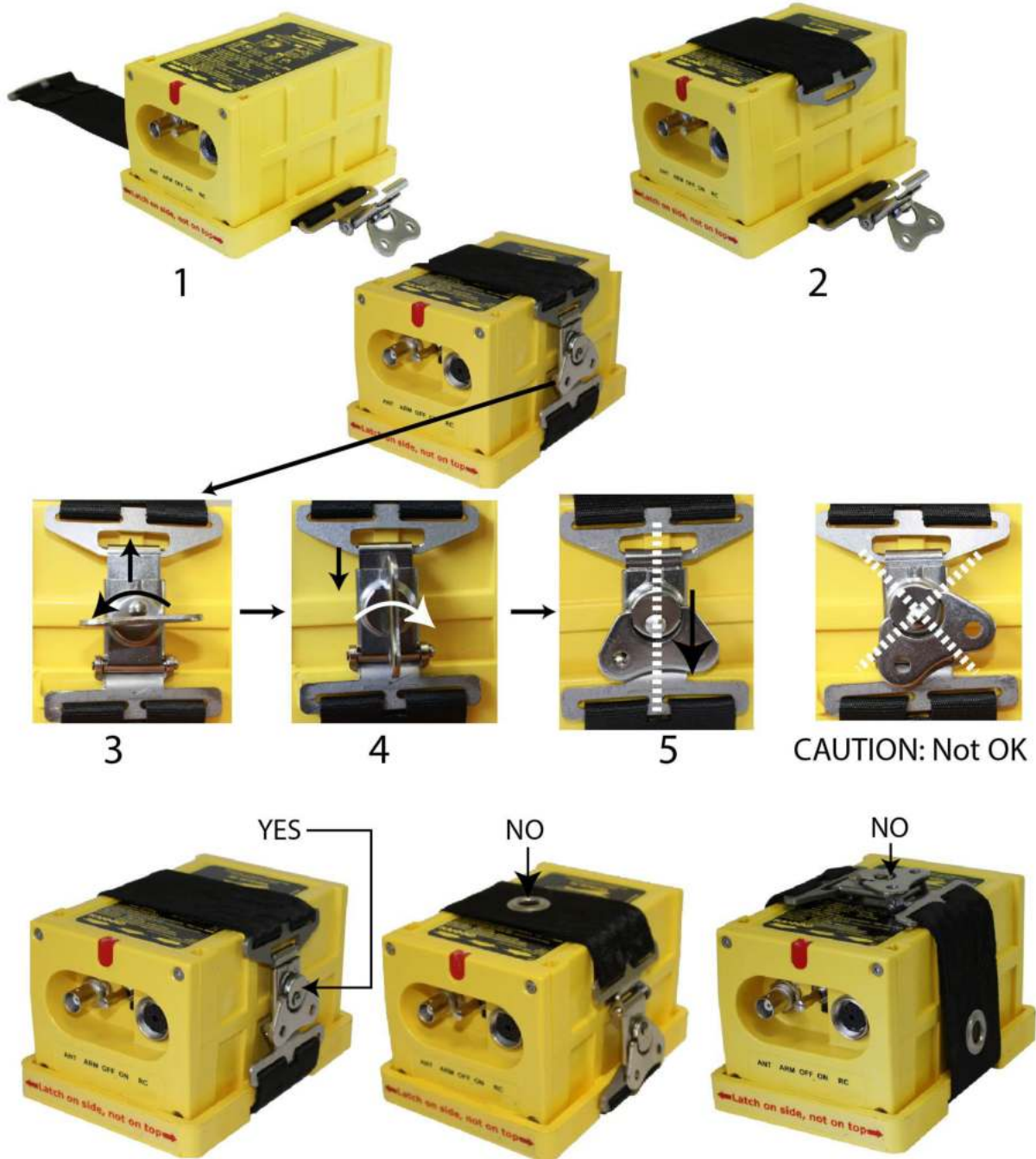
Figure 22: ELT Installation with Mounting Bracket INTEGRA AF P/N S1850551-04
