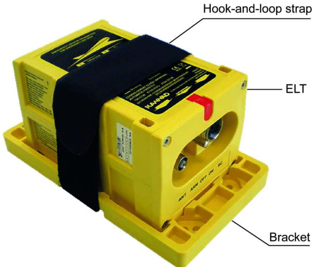
Figure 4: INTEGRA ELT with Mounting Bracket P/N S1840502-02
