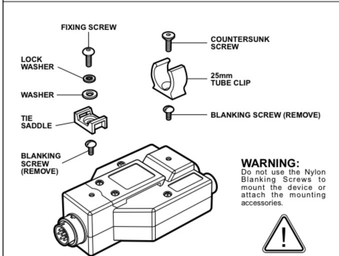
Depending on the application, small devices may be mounted permanently using Velcro, Screws, Tube Clips, or Cable Tie Saddles.
