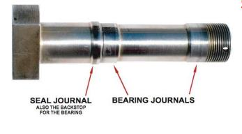
Cessna Axle on left is a casualty of bearing rotational wear Cause: Deficient Conventional Axle Nut
