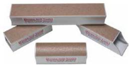
These user friendly sanding blocks are made from extruded, anodized aluminum. The 32mm (1.25") Radius Curve is covered on the external and internal radius with Tungsten Carbide abrasive sheets. The Contour Blocks come in either the Coarse (60US grit approx.) or Fine (120US grit approx.) Small block is 5.5" long and large block is 11" long. Benefits:
