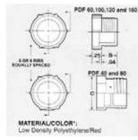
Series PDF plugs are designed for easy mechanical or hand installation on flat-faced O-ring fittings.
