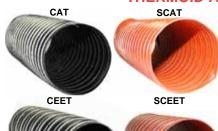
"CAT" - "CAT" type flexible hot or cold air ducting is extremely lightweight and highly flexible. Short lengths can be joined together to form a continuous length. Made of a single ply black neopreneimpregnated fiberglass with a spiral copper coated steel wire inside and wrapped with fiberglass cord on the outside. Suitable for conveying tumes and air a temperatures from -65° to over 350°F. Not recommended for handling liquids or highly abrasive materials, or for negative pressure applications.
