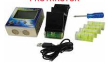
The Protector is a precision, highly accurate and simple to use device for checking, setting or changing propeller pitch. The resolution and repeatability is 0.05 degree and the accuracy is +/- 0.1 degree. It is powered with a standard 9 volt battery with approximately one year use life. P/N 12-04974
