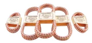
An endless elastic ring composed of multiple strands of natural rubber, wound into a circular skein. Braided cover is high grade yarn. Manufactured to meet specification MIL-C-5651B, Type II. Shock cord is used in landing gear to reduce shock transmitted to fuselage while landing and taxiing and on other shock mounting applications. Color coded to insure fresh stock.
