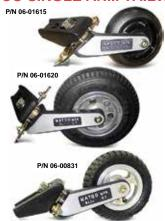
Matco tailwheels use a fiberglass reinforced nylon wheel with an operating load of 450 lbs. It takes over 5000 lbs to fail the wheel and it will hold up in the most rigorous conditions. Can be used with 1-1/4" or 1-1/2" leaf spring. These tailwheels are steerable, and are available with a 6 inch hard rubber solid tire or with 8" Shin pneumatic tire and tube for heavier aircraft. Tailwheel construction is anodized aluminum. Weight: 5 lbs.
