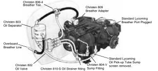
This accessory kit for Lycoming engines provides normal engine lubrication with minimal oil loss during aerobatic flight. It functions as a selfcontained extension of the normal engine oil and breather systems. Can be installed in a few hours without engine disassembly.
