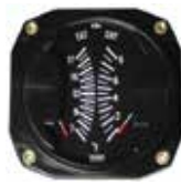
COMBINATION EGT & CHT 3-1/8" size, Wt.10oz., 700-1700°F/ 100-800°F. P/N 3DA1.....--- Order 1 EGT probe & 1 thermocouple.
