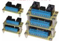
AE Relay Boards - Better than the Competition. These relay contacts are protected against inductive sparking generated from relays switching inductive loads such as motors and solenoids. The relay coils are also protected. This prohibits the relays from early failure. This also protects the switch contacts that drive the relay coils from failure.
