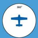
strobe light system must project light 360° around the aircraft's vertical axis. One or more strobe lights can be used.
