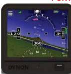
D3 lets pilots supplement their unreliable legacy instrumentation with an affordable, portable electronic attitude indicator that works. The D3 features the same reliable, proven AHRS engine from Dynon's bestselling panel-mounted products for experimental, light sport, and type certificated aircraft.
