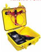
AIRCRAFT STATIC TEST ADAPTER
