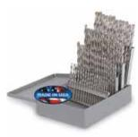
60 pc. Bright - Jobber Length - 118° Point - Wire Sizes - 95090850. Excellent general purpose drill bit. Precision CNC machined for faster, more efficient chip removal. Industrial-Grade NAS High Speed Steel (HSS). Heavy duty metal storage case. Numbered metal tip-out indexes keep bits organized. Made in the USA. Material applications: aluminum, copper, wood, plastic Size range: Wire #1-#60 .... P/N 12-04760
