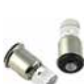
LED MIDJET FLANGED BI-POLAR LAMP T1-3/4 (5-28 VOLTS) Replaces miniature lamps: # 328, 345, 350, 7335 (5/6V), 330, 382, 394 (12/14V), 327, 376, 387 (24/28V). Attention: Not intended for use with Post Light Assemblies P/N 11-09629
