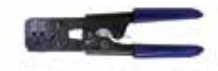
Crimps Seal-All terminals and seals in one cycle. Features two double Cavities, an orientation block and a ratchet mechanism to ensure that each crimp cycle is completed. Factory calibrated to be used only with Seal-All terminals and seals. Wire range 20-14. Pro Seal-All Crimper P/N 11-06593
